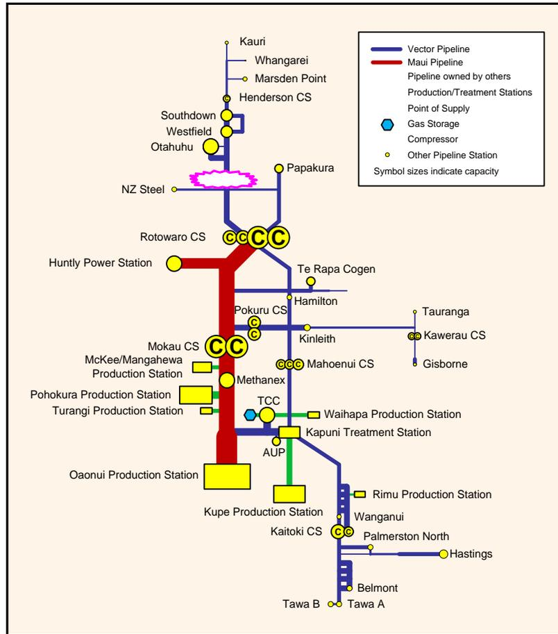
As can be seen from the schematic, there are no pipelines that bypass the damaged and isolated section. As a result, and due to the small amount of linepack in the north system, very rapid curtailment would be required so as to ensure that the distribution networks in Auckland and points north did not become depressurised.
